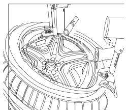
Note: When you mount/ demount the tire, tire rotates clockwise. If the tire is jamming during the process, please stop working and counterclockwise rotate the tire to remove the jamming.
