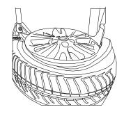
If the hook moves downwards, it may damage the tire.
