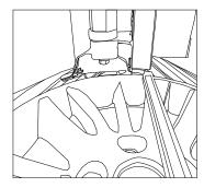
bead. Which can cause decoupling. So it is difficult to hook out the edge of the tire/ We suggest to rise up the lower bead. This can help hook out the bead.
