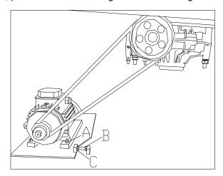
If the tool head is not locked or not located at the position 2-3mm higher than the rim, it is necessary to adjust the adjusting nuts A and B at the front end of hexangular shaft lock plate.
