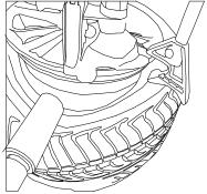
When mount upper bead, at the left side of the tool head, use the tire press to press
