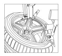
To protect the rim, it is required that the plastic cover for the tool head should be once two months. If damaged, these plastic parts should be changed at once.
