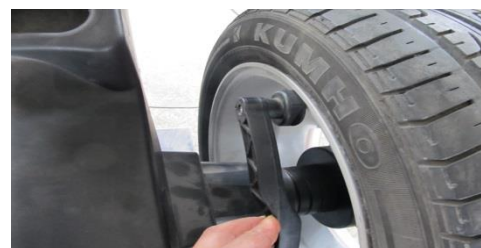
Pull the scale head at the third step of the internal measuring scale
