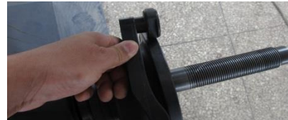
The scale head should be pressed on exterior eaves of the matcher
