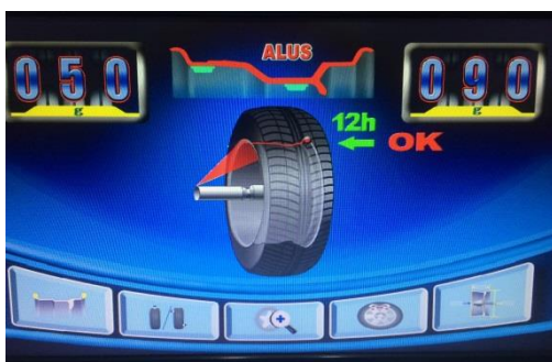
Confirmation of 12-Point Phase Position of Unbalance at Outer Side
