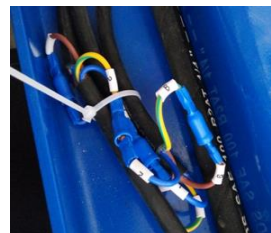
Line connection assembly, connected with the same number
