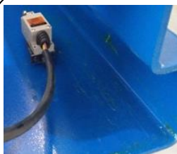
Travel switch (limit) installation diagram
